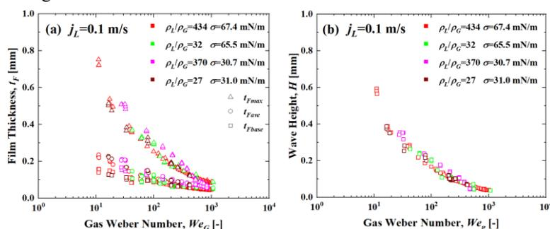
Fig. 1 Comparison of (a)  $t_{Fave}$  and (b)  $H$  against  $We_G$  under  $j_L = 0.1$  m/s.
