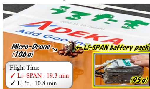
Fig. 2. Drone flight with the Li-SPAN battery pack.
