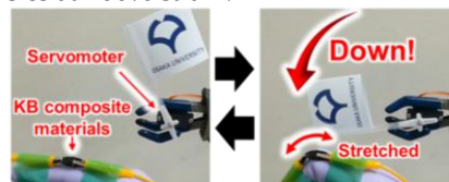
Fig. 4. Circuit and Photographs of stress-strain sensor and remote actuating system.
