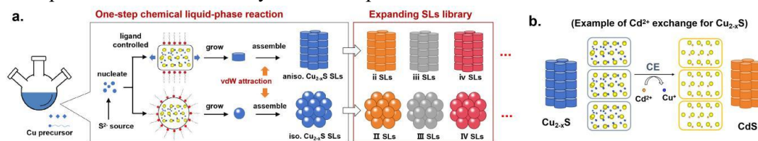
Fig.1 (a) Scheme of one-pot synthesis method of NC SLs and expansion of SLs species via CE, (b) preservation of crystallographic arrangement in the \text{Cd}^{2+} cation exchange.
