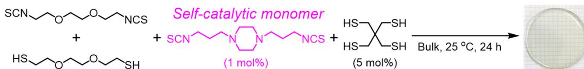
**Scheme 1.** Synthesis of networked polydithiourethane (NPDTU) with self-catalytic monomer.
