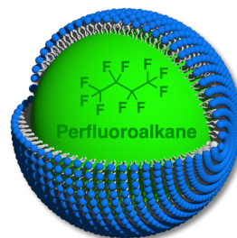
Fig. Schematic illustration of a microbubble formed by phospholipid and perfluoroalkane.
