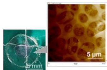
Figure 1. A cell-encapsulated device and an AFM image of triple-layered PPN equipped in the device.
