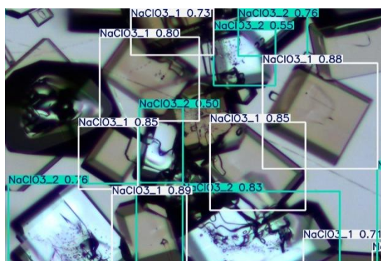
Figure 1. The detection image of sodium chlorate.
