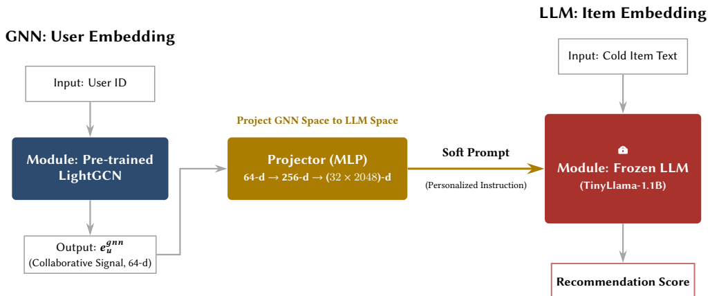
Figure 1: The overall architecture of GLCSRec. The process begins with a pre-trained LightGCN (Left) for extracting high-order user embeddings, followed by a multi-layer projector (Middle) that aligns these signals with the LLM input space. Finally, the Soft Prompts (Right) act as personalized instructions to guide the frozen LLM for item cold-start recommendation.
