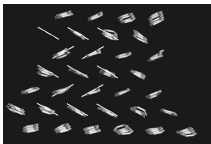
Fig. 10 Comparison of the structures found in Figs. 8-9 (orange) and an experimentally formed crystal structure of pentacene (white). Both have herringbone structures
