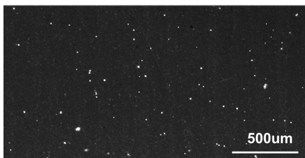
Fig.4 Optical microscope image of fogging toners on ITO substrate at application of DC voltage
