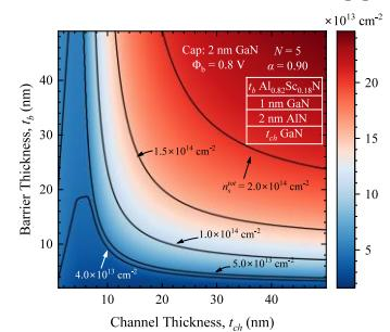
Figure 3: Contour plots of total 2DEG density as a function of channel and barrier thickness for 5-channel AlScN/1nm GaN/ 2nm AlN/GaN.
