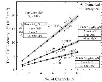
Figure 2: Total 2DEG density versus the number of channels for GaN-based heterostructures, calculated using the equations in Fig. 1. The numerical calculations were done with nextnano [3].
