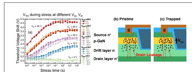
**Figure 1:** (a) Threshold voltage instability detected during OFF-state experiments with different gate voltages; (b/c) Charge trapping model.
