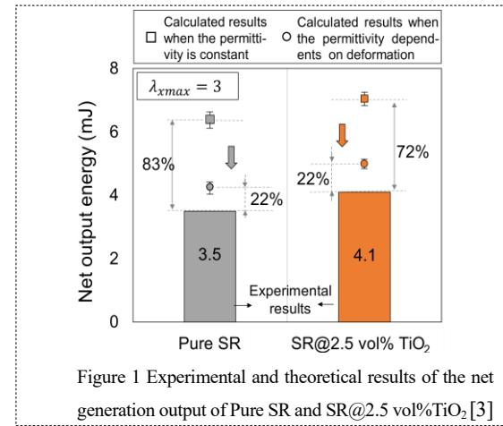
Figure 1 Experimental and theoretical results of the net generation output of Pure SR and SR@2.5 vol%TiO<sub>2</sub> [3]
