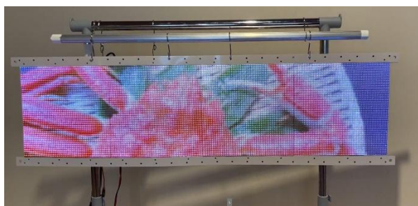
Fig. 3 A picture of the scalable flexible mini-LED panel (30 cm x 120 cm )
