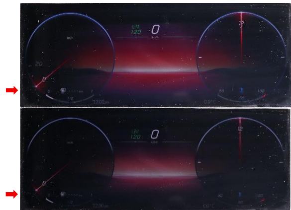
Fig. 5 A locally dimmed automotive HMI with (top) and without image enhancement (bottom).
