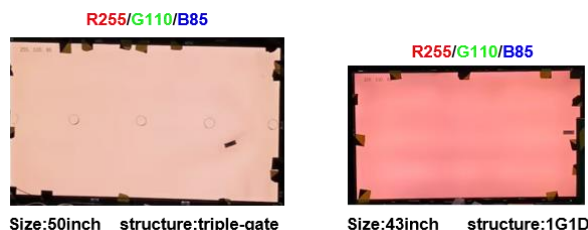
Fig. 1 Trigate skin color distortion phenomenon under different pixel architecture
