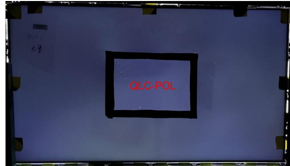
Fig. 10 The dark state of the wide-angle and normal polarizing films causes a whitening effect (the center is the wide-angle polarizing film, the periphery is the normal polarizing film, and the middle position is much better than the periphery).
