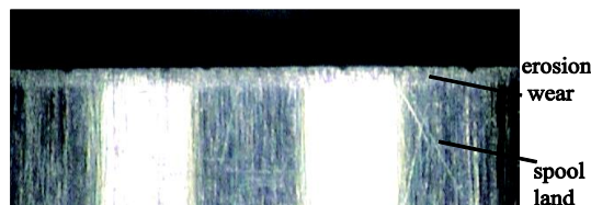
FIGURE 3. Photo of the Worn Spool Metering Edge after the Life Test (case 2)
