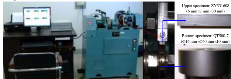
Fig. 1 Wear measurement apparatus of type MMS2A and specimen
