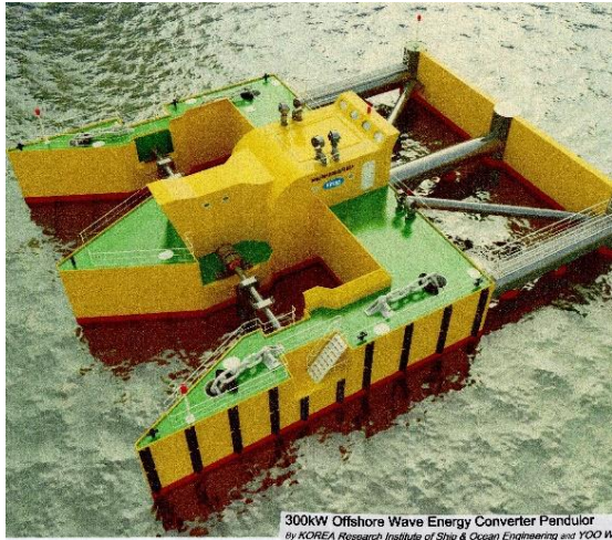
FIGURE 1 Floating Pendulum 300kW, Refined by, KRISO & YOOWON, Korea, (7) (original one Jap. Patent, 4448972, 2003) (5)
