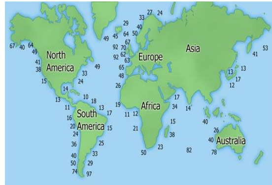
FIGURE 2 Wave power distribution in the world with the unit kW/m, (US Dept. of ENERGY)
