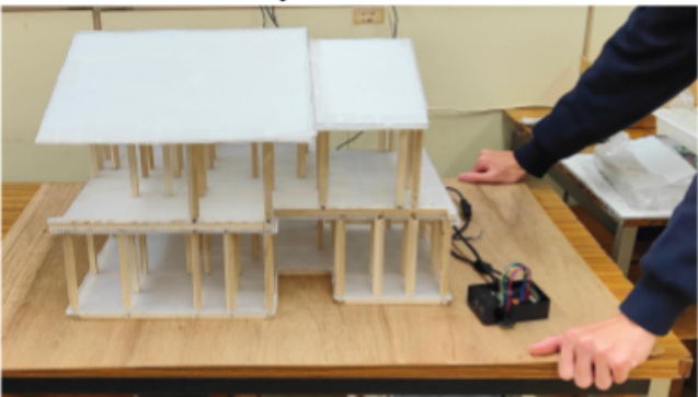
(図9) 模擬地震実験の様子 (Fig9) Simulated earthquake experiment
