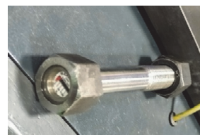
Fig. 4 Axial force indicator bolt
