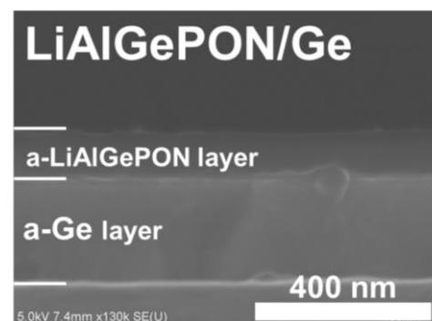
Fig.2 SEM image of LiAlGePON/Ge multilayer anode film
