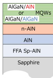
Fig. 1 Schematic image of sample structures of MQWs.
