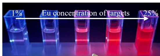
Fig. 1: Picture of the microparticle samples dispersed in ethanol under UV illumination.
