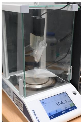
**Figure1.** Automated powder dispensing machine and electronic balance
