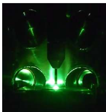
Figure 2: Arc-melting in automatic motion.
