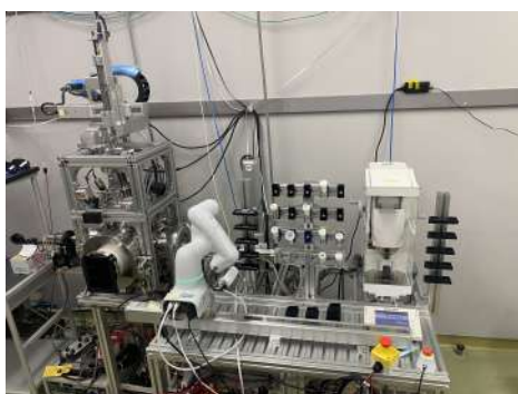
Figure 1: Automated arc-melting system.
