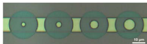
Fig. 1 Optical microscope image of Ge microdisk resonators with diameters of 3, 4, 6, 8 \mu\text{m} .
