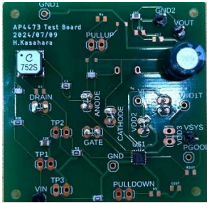
Fig.2 The layout of the evaluation board.
