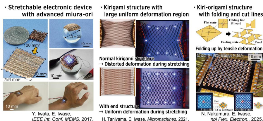
Fig. 1 Stretchable electronic devices using origami/kirigami/kiri-origami structure
