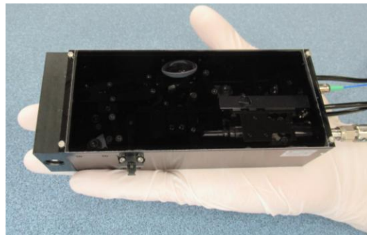
Fig. 1. Photograph of the developed palm-sized all-in-one BW-TPO module.
