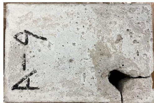
Fig.3 Crushed Test Piece
