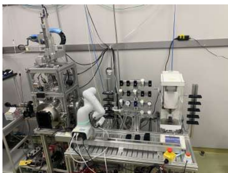
Figure 1: Automated arc-melting system.
