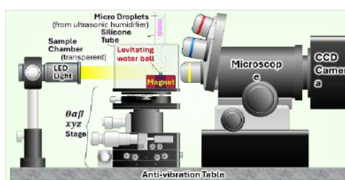
Fig. 2 Schematic diagram of magnetic levitation device
