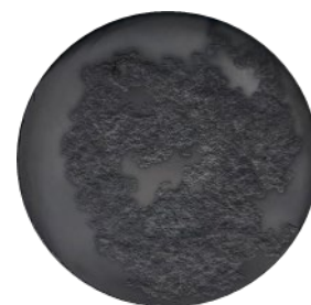
Fig.2 Erosion of graphite cathode (50 mmφ) when I_{oc} = 2.5 A.
