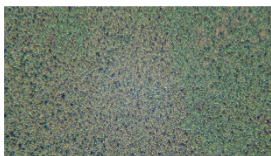
Fig. 1. Ge surface after chemical oxidation by using HNO 3 .
