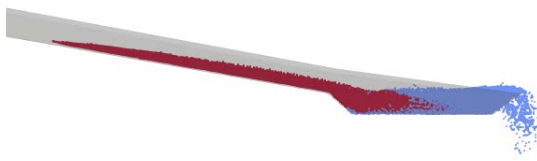
Fig. 2 Simulation results of the debris flow with \tau=60 Pa and \eta=0.3 Pa·s.
