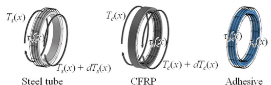
Fig. 2 Force equilibrium of each member in an infinitesimal element dx .
