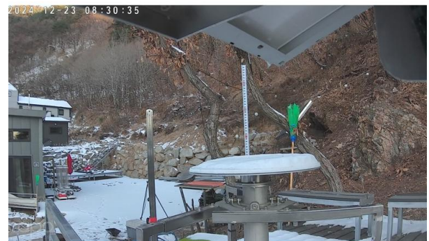
Fig. 1 Field measurement of snow depth and snow load
