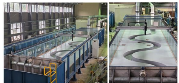
Fig. 1 Compound meandering channel experimental facility.
