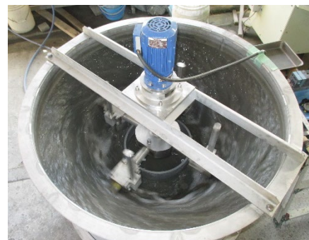
Fig. 1 回転式水中摩耗試験 Rotary underwater abrasion test
