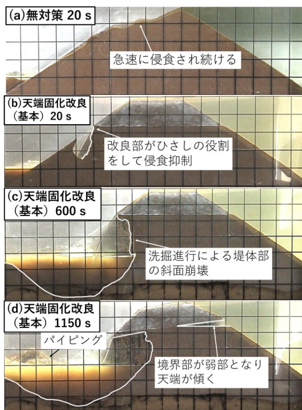
Fig. 3 越流開始後の侵食状況 Erosion progress after overtopping
