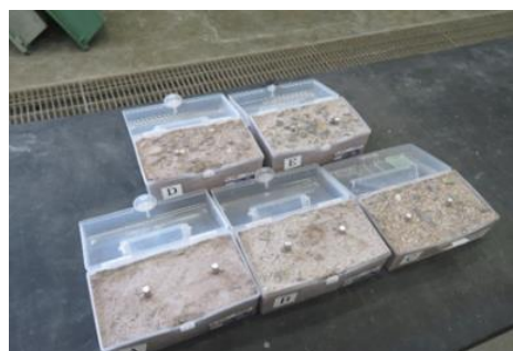
Fig.1 粗度調整供試体 Roughness-adjustable specimens
