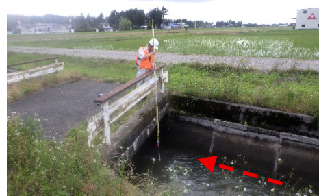
写真 2 電磁流速計の観測状況 Photo2 Electromagnetic Flowmeter Measurement Situation
