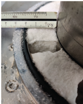
(c) A photo of an experimental shear zone in fine halite particles (thin)
