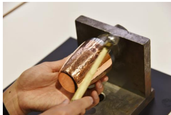
Hand-on of hammering of pure copper tumbler
