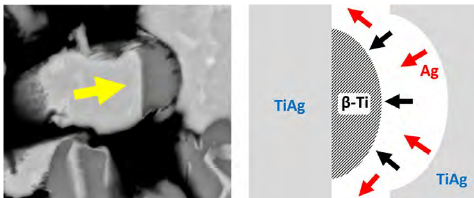
Fig. 1. Schematic of the liquid film migration mechanism.
